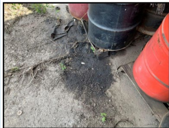
Photograph 4: Stained soil adjacent to drums under canopy.
